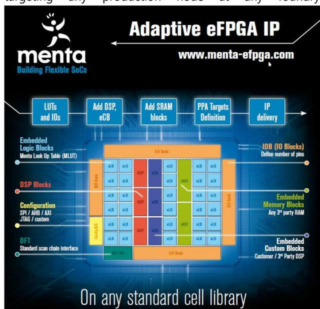
**Menta standard-cell based approach enables engineers to rapidly port the eFPGA to whatever new process geometry/variant they need** – Even in industrial and rad-hard grade versions. In addition, Menta IPs are fully verifiable in the customer's DA environment, and are designed to address various markets and applications.
